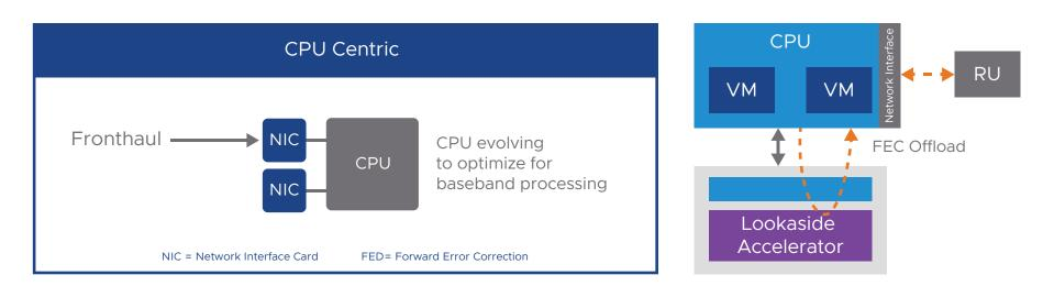
Lookaside processing is designed to address complex operations that require significant computational power. When a CPU encounters a computationally intense task, it offloads the task to the lookaside accelerator. The lookaside accelerator can then concurrently process the complex tasks while the primary CPU continues its standard operations, thereby optimizing overall system performance.
