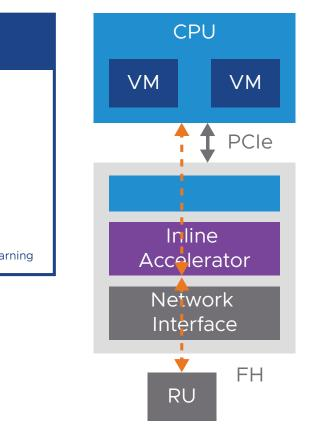
When data packets are routed through the network, inline accelerators immediately process the data, eliminating any potential lag or latency. By directly handling every packet, inline accelerators ensure quick responses and streamline operations, contributing to the overall network performance.
