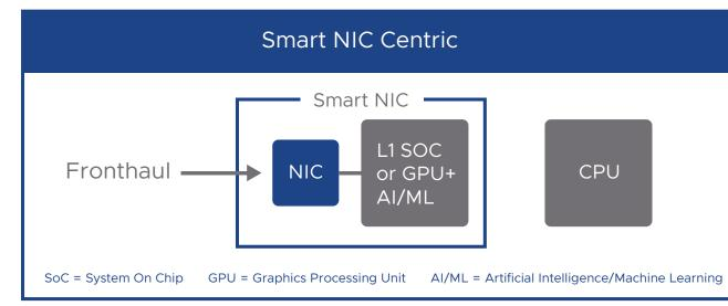
The term 'inline,' therefore, refers to the fact that these accelerators are within the main data path. While other accelerators may operate independently or on the side, inline accelerators are embedded directly within the data flow. They potentially interact with every data packet passing through the network, promoting swift processing and immediate data availability.
