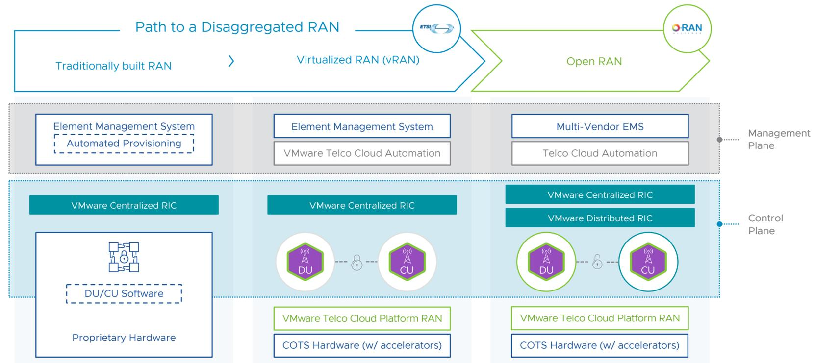
**Figure 4:** VMware Centralized RIC and VMware Distributed RIC
