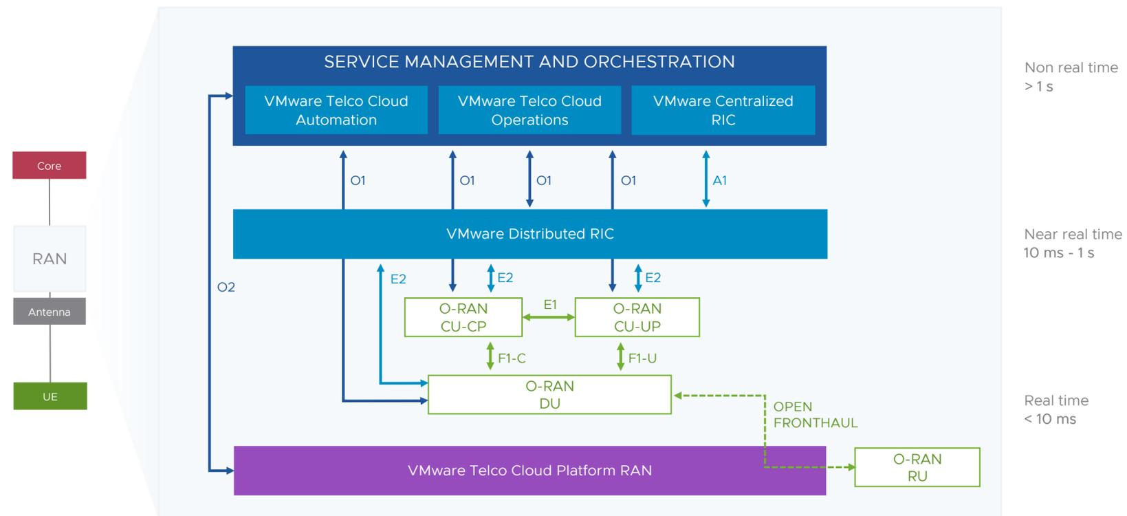
**Figure 3:** O-RAN architecture, now featuring VMware Centralized RIC, Distributed RIC and other VMware Telco Cloud offerings.
