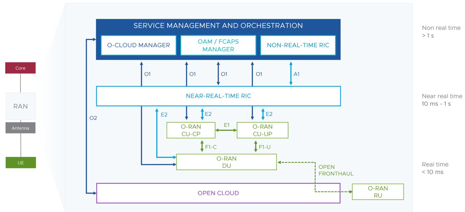
**Figure 2:** O-RAN Reference Architecture for Open RANs
